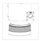
5 Pull the dust bag over the bag holder and close the bottom of the dust bag with a cable tie.
