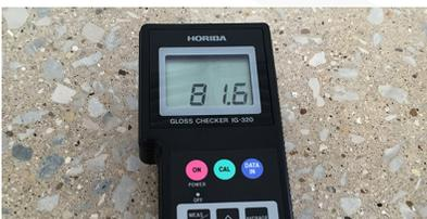
81.6 Gloss Meter reading of polished concrete after using the EGT Diamond System
