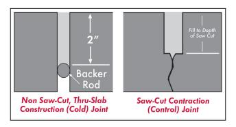
In construction (formed) joints that are not saw-cut, **Edge-Pro 90** should be installed at a minimum 2" depth. **DO NOT USE COMPRESSIBLE BACKER ROD IN STANDARD SAW-CUT CONTRACTION/CONTROL JOINTS!** Rod may be used 2" down in construction or saw-cut joints exceeding 2" in depth ONLY.
