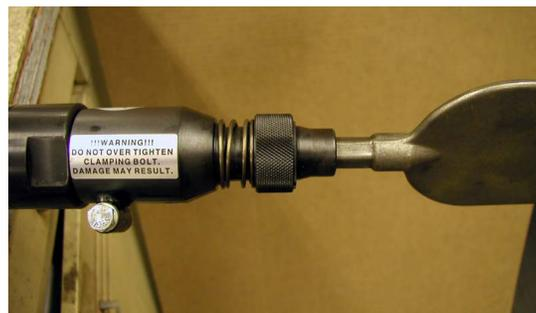
Pictured above shows the chisel installed. To remove a chisel reverse the above procedure and pull the chisel out of the chisel holder.
