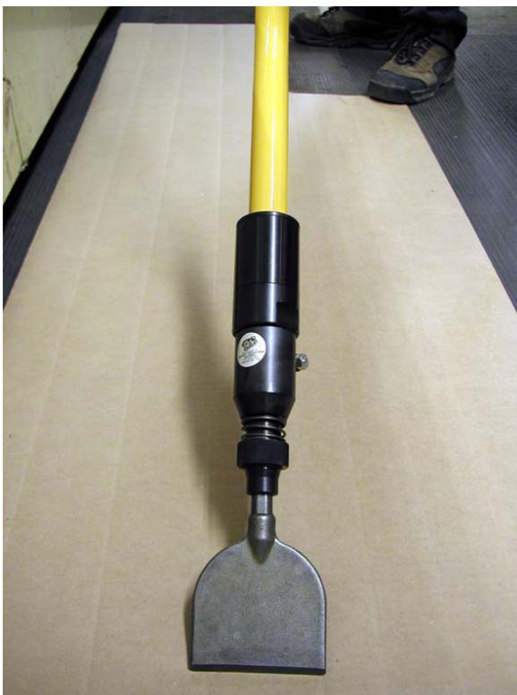
Be sure the chisel is oriented correctly. When in the operating position the straight flat edge should be closest to the work surface and the beveled edge should be facing up as shown in the photo above.
