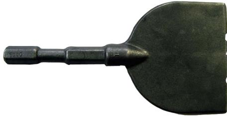
This is an example of a chisel that has been abused, probably hitting inserts, studs or other objects embedded in the working surface. To get maximum life out of a chisel be careful when working around objects protruding out of the work surface.
