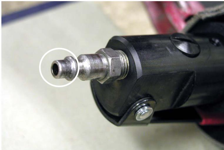
To lubricate the ALR put four (4) to five (5) drops of light weight machine oil in the hose connector circled above before connecting the air supply, graphite oil in extremely cold weather.
