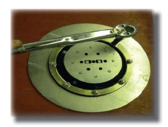
Final assembly as viewed from the main mounting plate side showing proper alignment of holes.
