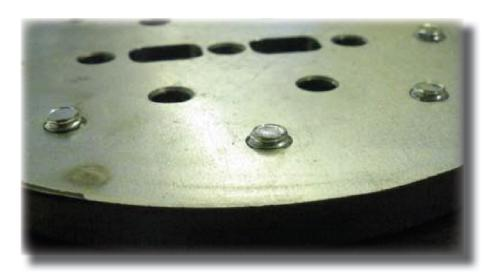
Note: The screw in the forefront is properly torqued while the screw to the left and right are over and under tightened respectively.
