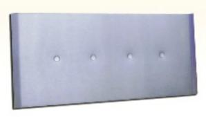
This blade is used when the concrete has begun to set. The blades are tilted from 3 degrees to 5 degrees and usually used at full speed. They make the concrete surface hard and glossy.
