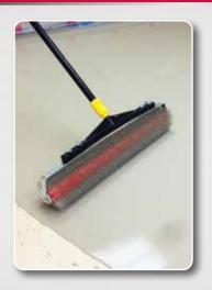
Designed for use with Rapid Set® TRU® Self-Leveling, and TRU® Gray Self-Leveling, and LevelFlor®. Closely spaced spikes are more effective at releasing trapped air in these fine aggregate self-leveling products without leaving a pattern in the finished surface.
